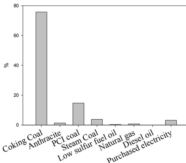
**Fig. 1.** Energy consumption profile of the mill A.
