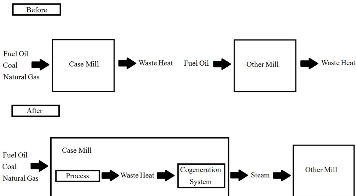
Fig. 6. Comparison before and after the construction of steam network in the mill A.
