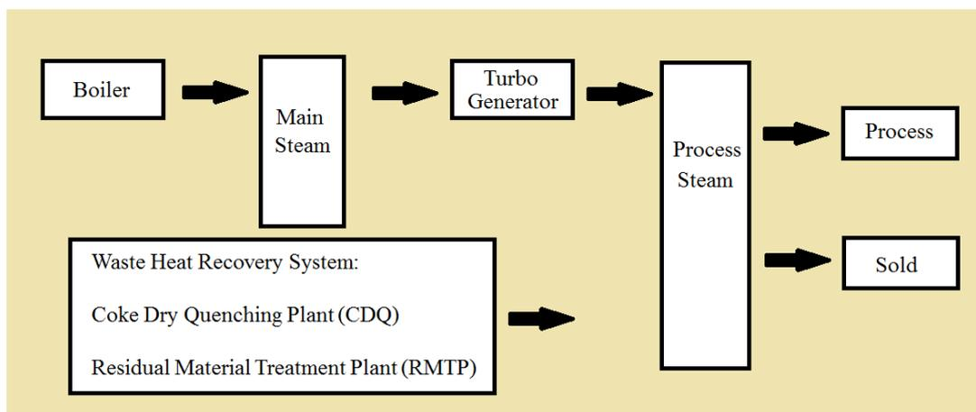
Fig. 5. Steam processing in the mill A.
