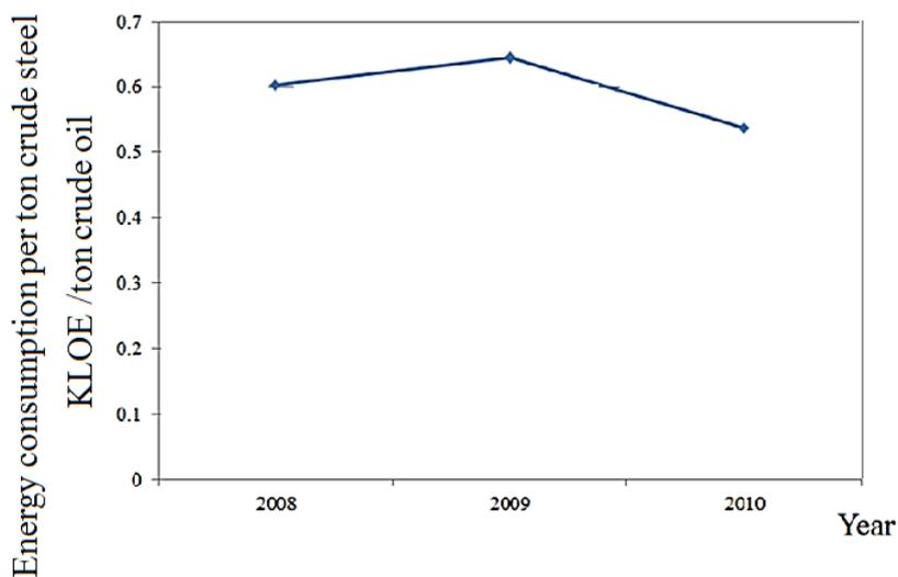
Fig. 3. Energy consumed per ton crude steel of the mill A.
